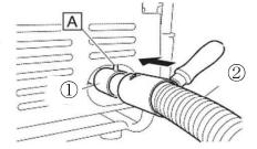
2. Fit notch **B**of exhaust pipe extension ② to boss **A** of muffler exhaust pipe ①.
