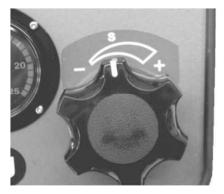
4. After a vacuum is produced, immediately return the priming lever to the original position, and stop the engine.
