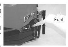
Air vent is installed on the fuel filler cap. Close the cap tightly after refilling.
