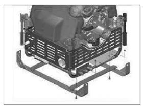
The TRANSPORTING DEVICE (TRANSPORT FRAME KIT) consists of the following parts.
