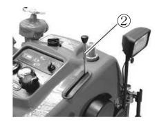
3. Operate the throttle dial to raise the pump pressure almost to 10 bar, and then check for water leaks from each part of the pump and the cooling water piping.
