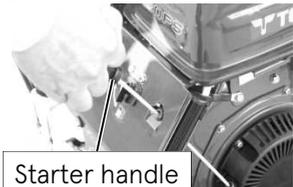
**NOTE** • To start the engine with manual starter, engage the manual starter ratchet by pulling the starter rope slowly. And then pull the starter handle quickly with great force from the position in which feeling harder resistance.
