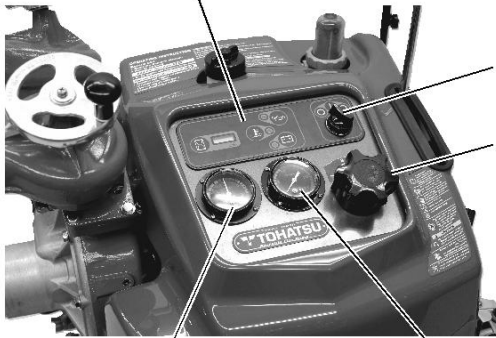
Pressure gauge for suction
