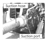
2. Start the engine, and lift the priming lever to run the vacuum pump.
