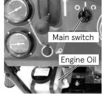
The engine remains operational for more than 30 minutes even after the buzzer sounds.
