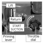
3. Operate the throttle dial to raise the pump pressure almost to 1 MPa (10 bar, 145 psi), and then check for water leaks from each part of the pump.
