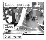
2. Turn the throttle dial to "START·SUCTION (S)" position. Start the engine. Lift the priming lever to run the vacuum pump, and check that the pressure gauge for suction indicates approximately -0.08 MPa (-0.8 bar,-12 psi). Return the priming lever to the original position.
