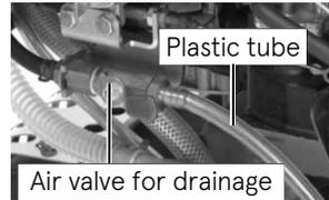
5. Insert the plastic tube in the container filled with antifreeze fluid.
