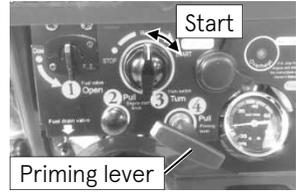
4. After a vacuum is produced, return the priming lever to the original position, and stop the engine.
