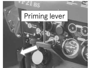
4. Operate the throttle lever to raise the pump pressure almost to 1MPa (145psi), and then check for water leaks from each part of the pump and the cooling water piping.
