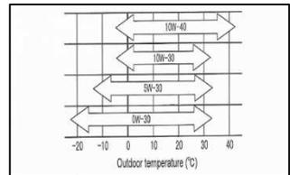
For operation in cold weather (10°C below or less), 0W-30 is recommender.
