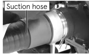
2. Place the end of the hose into the water more than 300mm (11.8in) deep from the water surface, and then close the discharge valve handle.
