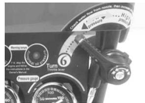
4. Turn the main switch to the “START” position. Release the main switch immediately after the engine started.
