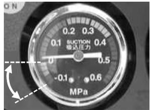
7. Open the drain valves slowly to expose it to the atmosphere, and check that the pointer of the pressure gauge for suction returns to "0".
