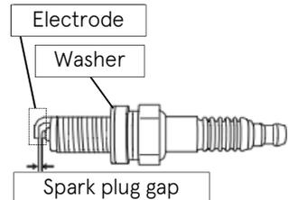
5. Assemble the spark plug as far as (a) by hand. Tighten the plug further to the specified torque using a plug wrench. (b)
