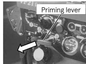
2. Check that the pumped water is discharged continuously from the priming outlet of the vacuum pump.
