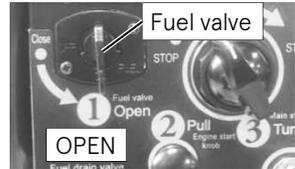
2. Turn the main switch to RUN position and pull the engine start knob.
