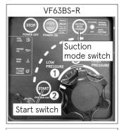
4. Turn the throttle dial to the suction position, then the pump will start to suck up water automatically.
