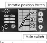
These lamps turn on when the throttle position is at "\$" position
