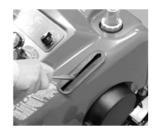
5. Check that the vacuum pressure of the pressure gauge for suction shows below -0.8 bar.
