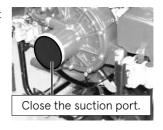
2. Pull the priming lever to run the primer (vacuum pump), and check that the pressure gauge for suction pointer reads approximately -0.8 bar.
