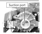
WARNING · Putting a finger or a hand into the suction port while the pump is running without installing the strainer, it may be seriously damaged by the rotating inducer.
