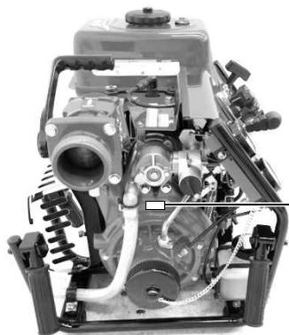
The pump identification number is marked on the pump case.
