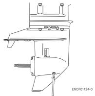
3. Insert the oil tube nozzle into the lower oil plug hole, and fill with gear oil by squeezing the oil tube until oil flows out of the upper plug hole and bubbles is disappeared to remove the air.
