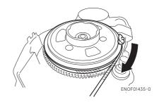
Tie a loop in the another end of the emergency starter rope and attach socket wrench that is included in the tool kit.
