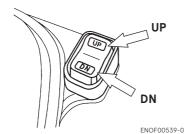
It is possible to tilt up or down in spite of main switch "ON" or "OFF".
