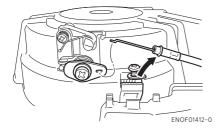
3. Remove the bolts (3 pcs) and remove the recoil starter.
