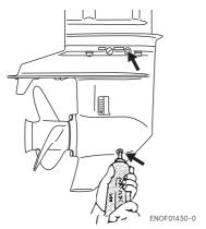
Install the upper oil plug, and then remove oil tube nozzle and install the lower oil plug.
