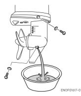
Insert the oil tube nozzle into the lower oil plug hole, and fill with gear oil by squeezing the oil tube until oil flows out of the upper plug hole and bubbles is disappeared to remove the air. ENON00033-0
