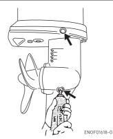
Install the upper oil plug, and then remove oil tube nozzle and install the lower oil plug.
