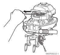
10. After engine starts, do not reinstall recoil starter and top cowl.
