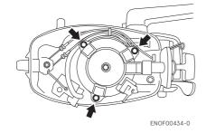
Insert the knotted end of the starter rope into the notch in the flywheel and wind the rope around the flywheel several turns clockwise.
