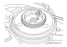
5. Tie a loop in the another end of the emergency starter rope and attach socket wrench that is included in the tool kit. ENOW00860-0
