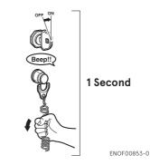
2. Within 5-10 seconds, pull the red knob on the safety switch out and release.
