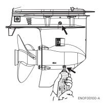
4. Install the upper oil plug, and then remove oil tube nozzle and install the lower oil plug.
