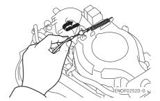
3. Remove the bolts (3 pcs) and remove the recoil starter.
