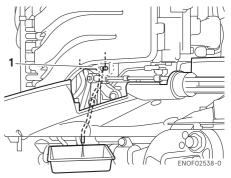
1. Vapor separator drain screw
