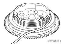
Tie a loop in the another end of the emergency starter rope and attach socket wrench, Both the loop and the wrench are provided in outboard motor box.
