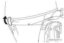
Remove starter lock cable from recoil starter by pulling the starter lock cable.
