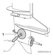
1. Gear case flushing device
