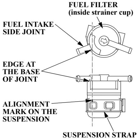
7. Install a new fuel filter. Assemble the fuel filter by aligning the edge at the base of the fuel intake side joint of the fuel filter with the alignment mark on the suspension as shown above.
