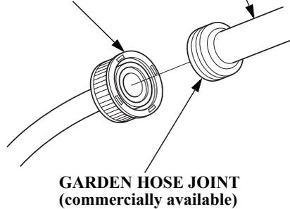
5. Screw the flush port connector onto the garden hose.
