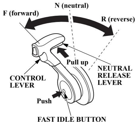
The fast idle button allows you to increase the idle speed without engaging the drive gears. Move the control lever toward the F (forward) or R (reverse) position after pushing in the fast idle button to increase the idle speed.
