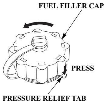
4. The fuel filler cap will lock again. Press down the pressure relief tab, and turn counterclockwise to remove the fuel filler cap.
