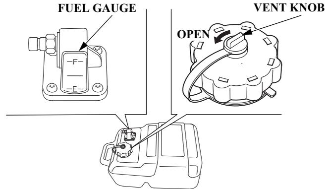
Check the fuel gauge and refill the tank when necessary.
