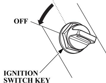
2. Turn the ignition switch key to the OFF position to stop the engine.
