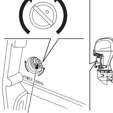
The outboard motor can also be tilted manually after opening the manual relief valve. This feature enables the outboard motor to be tilted up or down when no battery is connected.
