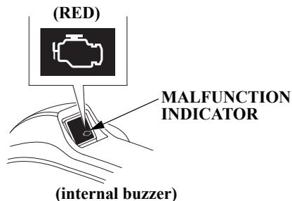
When the engine control system detects an engine control system malfunction, the malfunction indicator turns on and the buzzer sounds at one-second intervals.
