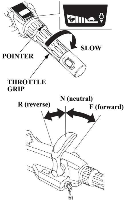
To shift gears, turn the throttle grip to the **SLOW** position; then move the gearshift lever to select the **F** (forward), **N** (neutral), or **R** (reverse) gears.
