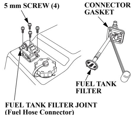
1. Remove the four 5 mm screws using a flat screwdriver, and then remove the fuel hose connector and fuel tank filter from the tank.
