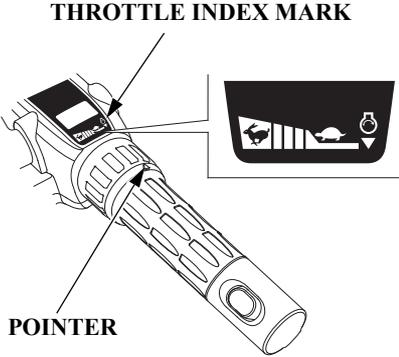
The throttle grip controls engine speed.
