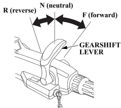
The gearshift lever is used to select F (forward), N (neutral), or R (reverse) gears.
