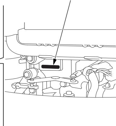
The frame serial number is stamped on a plate attached on the right side of the stern bracket.
