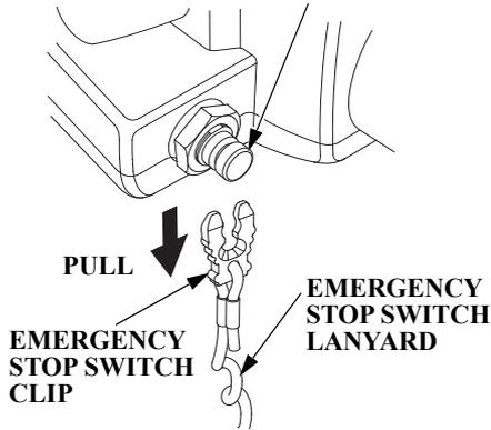
To stop the engine in an emergency, pull the emergency stop switch clip out of the emergency stop switch by pulling the emergency stop switch lanyard.
