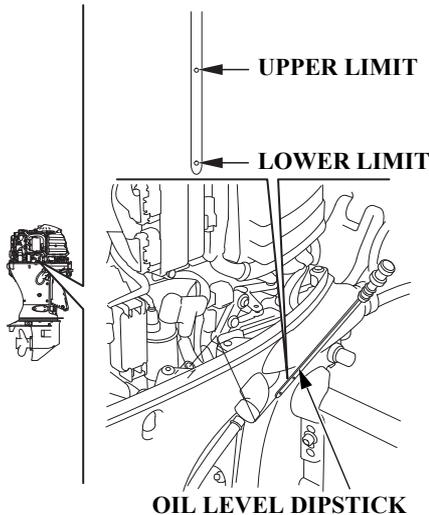
3. Insert the dipstick all the way in, and then remove it and check the oil level shown on the dipstick.
