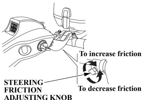
Tighten the steering friction adjusting knob securely.
