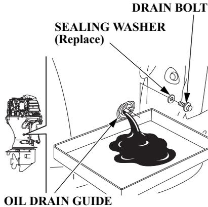
2. Place a suitable container below the oil drain guide to catch the used oil, and then remove the oil filler cap (p.96) and the drain bolt.
