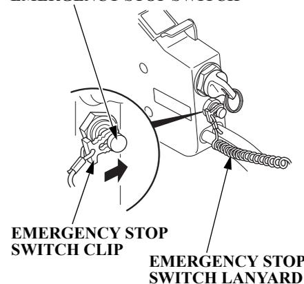
1. Put the emergency stop switch clip in the emergency stop switch, and securely to the operator or to the operator's PFD (Personal Flotation Device).
