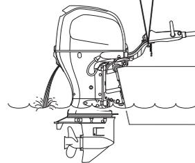
Install the height adjustment block so that the selected angle of the tiller handle is in this position.
