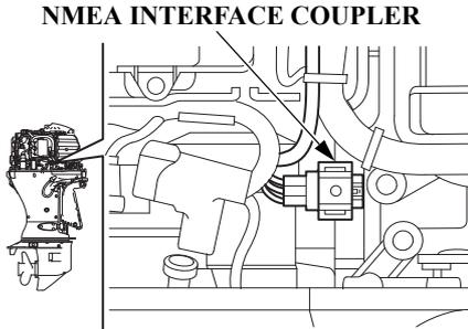
The NMEA2000<sup>®</sup> interface coupler can provide information regarding engine speed, fuel consumption, and various warnings to an existing NMEA2000 network via an optional interface cable. Contact your dealer for more information.
