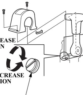
Adjust the control lever friction adjuster so the control lever will hold a constant throttle setting while cruising.
