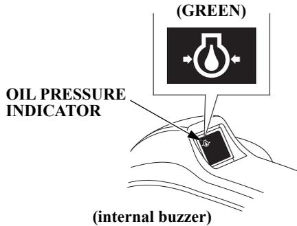
When the oil pressure indicator is lit, oil pressure is OK.
