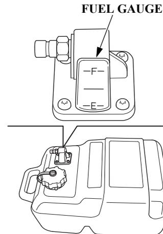
A fuel gauge is built into the fuel tank connector of the portable fuel tank.
