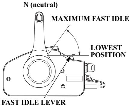
The fast idle lever allows you to increase the idle speed only when the control lever is in the N (neutral) position. Place the fast idle lever in its lowest position to cancel the fast idle and return the control lever to normal operation.
