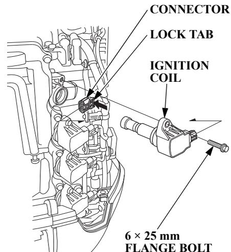
4. Remove the 6 × 25 mm flange bolt. Disconnect the connector by pushing the lock tab and remove the ignition coil.
