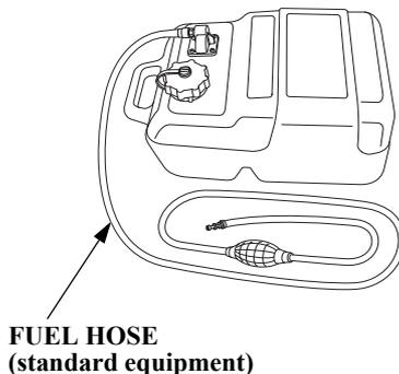
Empty the portable fuel tank into an approved gasoline container. Use a funnel to avoid spilling fuel. Rinse the fuel tank with nonflammable solvent to remove any accumulated sediment.
