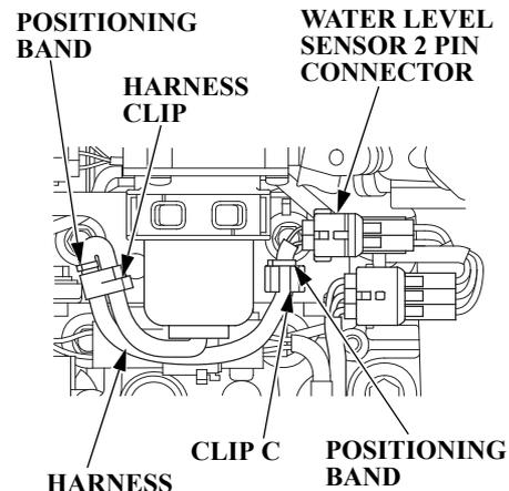
10. Connect the water level sensor 2 pin connector. Install the harness to clip C and the harness clip. Align the positioning bands on the harness with the end of clip C and the harness clip as shown above.
