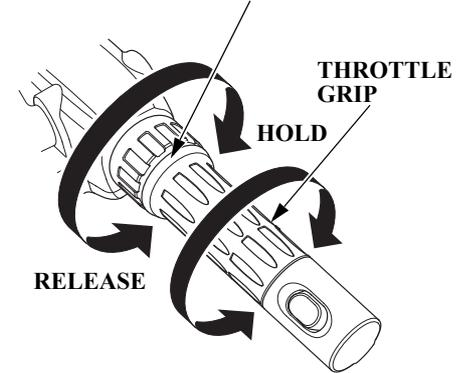
Use the throttle friction adjuster to help hold a constant throttle setting while cruising.
