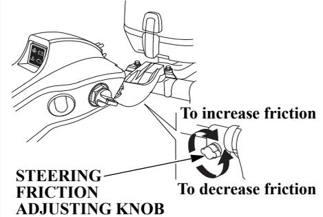
Use the steering friction adjusting knob to help hold a steady course while cruising.
