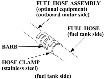
1. Remove the hose plug from the outboard motor side fuel hose. Insert the fuel hose joint into the outboard motor side fuel hose and secure it with the hose clamp (p.56).
