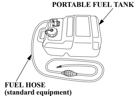
The portable fuel tank has a capacity of 6.6 US gal (25 L) and has a fuel gauge built into the fuel tank connector.
