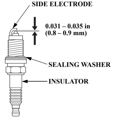
7. Measure the spark plug electrode gap with a wire-type feeler gauge. Correct the gap, if necessary, by carefully bending the side electrode. The gap should be: 0.031 - 0.035 in (0.8 - 0.9 mm)
