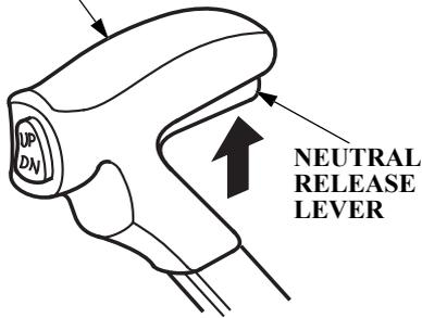
The gearshift/throttle control lever controls engine speed and selects F (forward), N (neutral), or R (reverse) gears.
