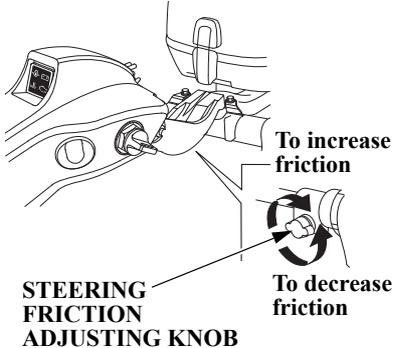
Use the steering friction adjusting knob to adjust the tiller handle friction. Turning it clockwise increases friction and turning it counterclockwise decreases friction.
