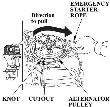
7. Set the alternator pulley so the cutouts are on the right and left sides of the alternator pulley as shown. Hook the knot at the end of the starter rope against a cutout in the alternator pulley, and wind the starter rope one and a half turns clockwise along the groove in the alternator pulley.
