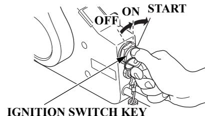
4. Turn the ignition switch key to the ON position; the buzzer will sound twice.
