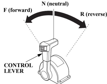
To shift gears, move the control lever to select the F (forward), N (neutral), or R (reverse) gear.
