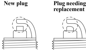
6. Inspect the spark plugs. Replace them if the electrodes are worn, or if the insulators are cracked or chipped.
