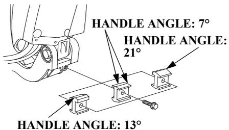
Install the height adjustment block so that the selected angle of the tiller handle is in this position.
