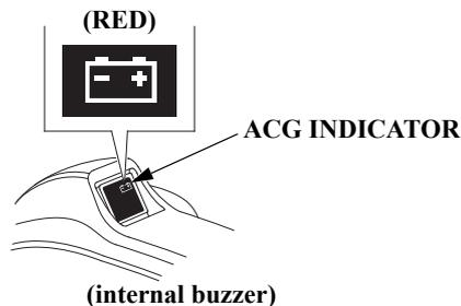
The ACG indicator turns on and the buzzer sounds in one-second intervals when the charging system is faulty.
