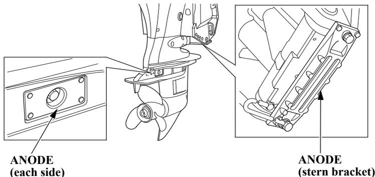
The anodes are made of a sacrificial material that helps to protect the outboard motor from corrosion.
