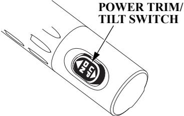
The power trim/tilt switch is located on the tiller handle or on the control lever. It is a rocker switch with UP and DN (down) positions for changing the angle of the outboard motor.
