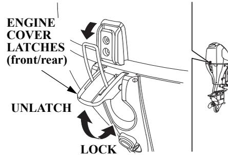
The engine cover latch fastens the engine cover to the outboard motor.
