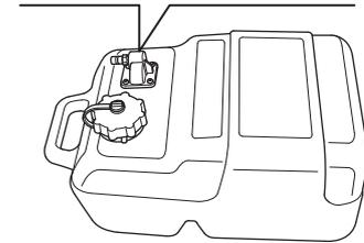
2. Connect the fuel hose to the tank and the outboard motor, as shown. Be sure both connectors snap securely into place. Always disconnect the fuel hose when storing or transporting the outboard motor.
