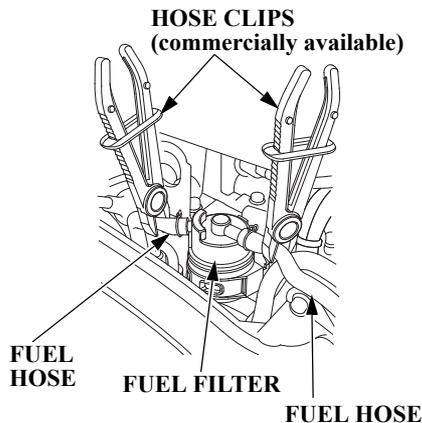
3. Before removing the fuel filter, to prevent fuel leakage, place fuel hose clips on the fuel hoses on each side of the fuel filter.
