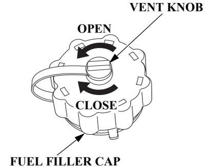
The fuel filler cap is provided with a vent knob to seal the portable fuel tank for carrying it to and from the boat. Open the vent by turning the vent knob counterclockwise all the way before starting the engine.
