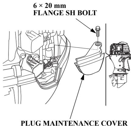
3. Remove the 6 × 20 mm flange SH bolt and remove the plug maintenance cover.
