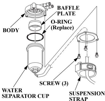
7. Remove the three screws and separate the water separator cup from the body.
