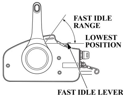
3. Leave the fast idle lever in the OFF (fully lowered) position.
