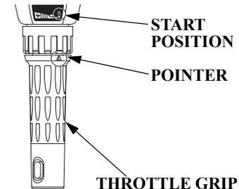
3. Align the engine start symbol "Ⓚ" on the tiller handle with the pointer "▶" on the throttle grip.
