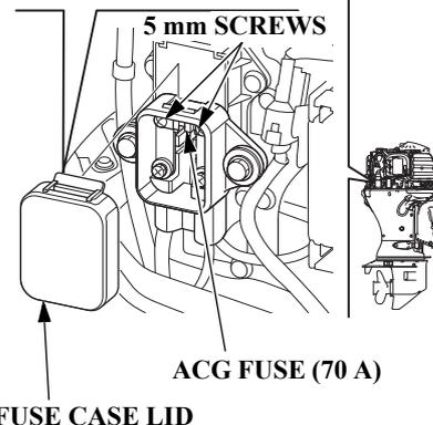
1. Stop the engine and disconnect the battery cable.
