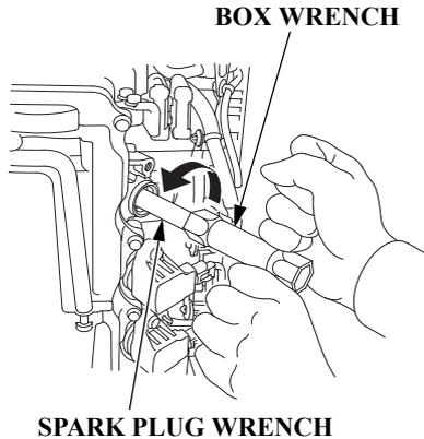
5. Remove the spark plug using the spark plug wrench, box wrench and the Phillips® screwdriver (accessories).
