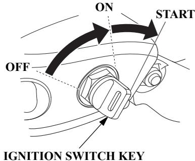
5. Turn the ignition switch key to the START position and hold it there until the engine starts. When the engine starts, release the key, allowing it to return to the ON position.
