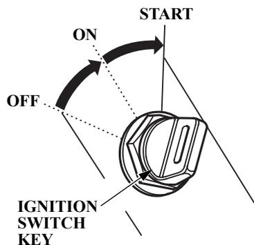
3. Turn the ignition switch key to the ON position; the buzzer will sound twice.
