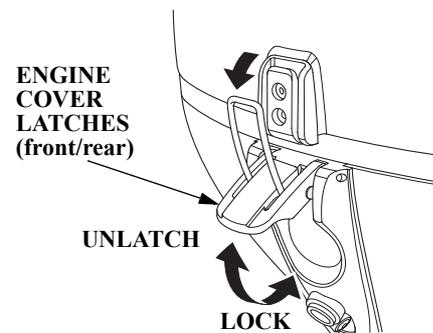
The engine cover latches fasten the engine cover to the outboard motor.
