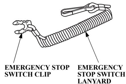
The emergency stop switch clip must be inserted in the emergency stop switch in order for the engine to start and run. The emergency stop switch lanyard must be attached to the operator's PFD (Personal Flotation Device) or to the operator securely.
