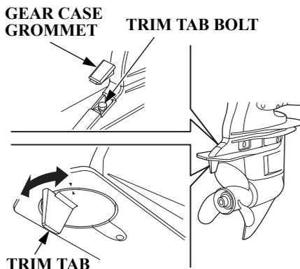
Adjust the trim tab with the engine stopped. Remove the gear case grommet. Loosen the trim tab bolt above the trim tab, turn the trim tab, and then tighten the bolt and install the gear case grommet securely.
