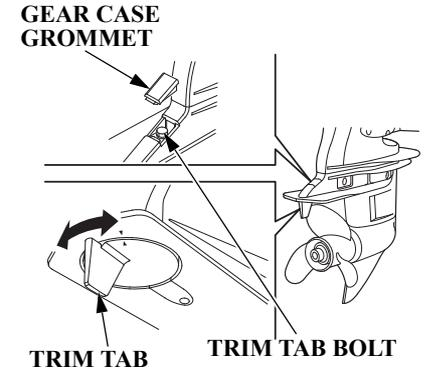
The trim tab compensates for “torque steer,” which is a reaction of the outboard motor to propeller rotation.
