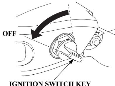
2. Turn the ignition switch key to the OFF position to stop the engine. In the event that the engine does not stop when the ignition switch key is turned to the OFF position, pull the emergency stop switch clip out of the emergency stop switch by pulling the emergency stop switch lanyard (p.72).
