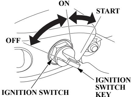
The ignition switch controls the ignition system and the starter motor.
