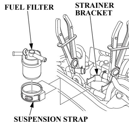
4. Remove the fuel filter assembly from the strainer bracket. If it is difficult to remove the fuel filter assembly by yourself, consult an authorized TOHATSU dealer.
