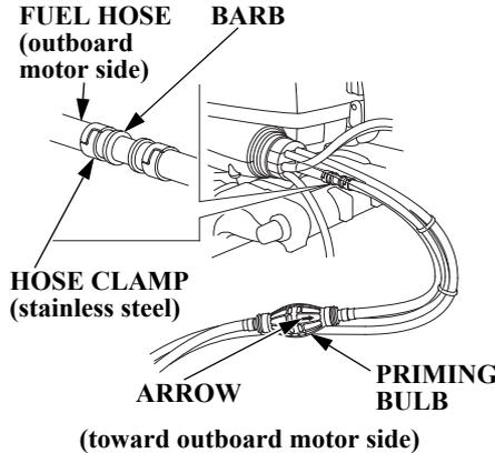
1. Remove the hose plug from the outboard motor side fuel hose. Insert the fuel hose joint into the outboard motor side fuel hose and secure it with the hose clamp. Make sure the arrow mark on the priming bulb points toward the outboard motor side.
