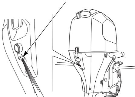
Water should flow from the cooling system indicator while the engine is running. This shows that water is circulating through the cooling system.
