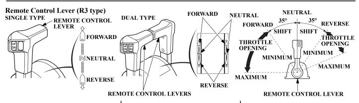
Shifting gear into forward, reverse, or neutral and the engine speed adjustment can be performed with the remote control lever.
