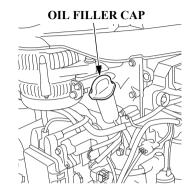
5. Reinstall the oil filler cap securely. Do not overtighten.
