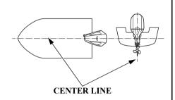
Install the outboard motor at the stern, at the center line of the boat.
