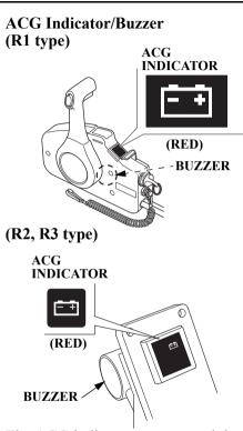
The ACG indicator turns on and the buzzer sounds when the charging system is faulty.
