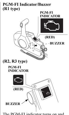
The PGM-FI indicator turns on and the buzzer sounds when the engine control system is faulty.
