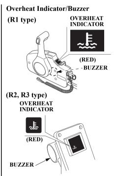
The overheat indicator turns on and the buzzer sounds when the engine cooling circuit is faulty. The engine speed slows down this time.
