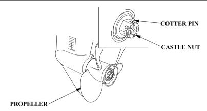
Engine speed varies according to the propeller size and the boat condition. Use of the outboard motor outside the full throttle speed range will adversely affect the engine and cause a serious problem. Use of the correct propeller assures powerful acceleration, top speed, excellency in terms of economy and cruising comfort, and it assures longer engine life as well.
