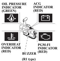
If the engine oil pressure drops and/ or the engine overheats, either or both warning systems could be activated. When activated the engine speed will decrease gradually and the green oil pressure indicator will turn OFF and the red overheat indicator will turn ON. A continuous buzzer will sound
