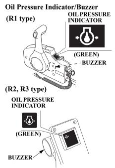
The oil pressure indicator turns off and the buzzer sounds when the oil level is low and/or the engine lubrication system is faulty. The engine speed slows down gradually this time.
