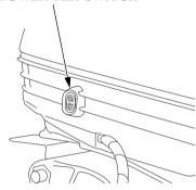
The power tilt switch located on the outboard motor pan is a convenience switch for tilting the outboard motor for trailering, or performing outboard maintenance. This power tilt switch should only be operated with the boat being stopped and engine off.
