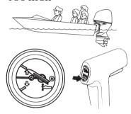
With the outboard motor trimmed high the trim meter will read as shown. To lower the bow decrease the outboard motor trim angle by pressing the DN (down) portion of the power trim/tilt switch.
