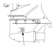
COOLING WATER INTAKE PORT (each side)
