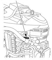
The engine serial number is stamped on the upper right side of the engine.
