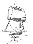
**COOLING WATER INTAKE PORT** (each side)
