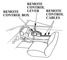
Install the remote control box in the position where is easy to operate the remote control lever and switches. Be sure that there are no obstacles on the route of the control cable.
