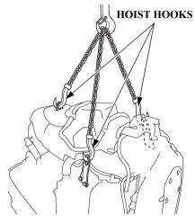
2. Set the hoist hooks against the lifting eyes and hang the outboard motor to remove it from the boat
