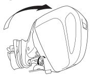
Tilt up the outboard motor using the tilt lock lever when mooring the boat. Shift the control lever into the NEUTRAL position and stop the engine before tilting up the outboard motor.
