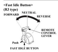
Use the fast idle button and the remote control lever to adjust the engine speed without gearshift when warming up the engine.
