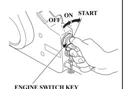
3. Turn the engine switch key to the START position and hold it there until the engine starts.
