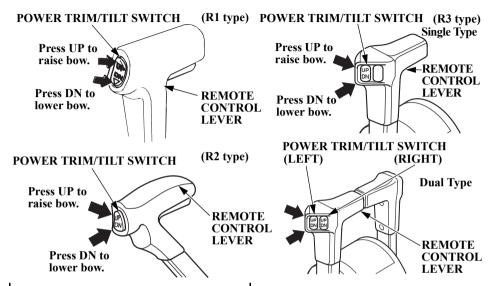
Consult an authorized TOHATSU Outboard Motor dealer for the method to adjust the tilt limit switch. Press either UP or DN (down) of the power trim/tilt switch and tilt the outboard motor to the best position in compliance with the cruising conditions.
