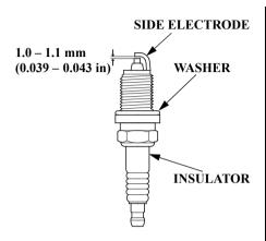
7. Measure the plug gaps with a feeler gauge. Correct the gap, if necessary, by carefully bending the side electrode.
