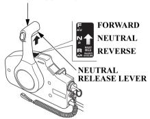
Shifting gear into forward, reverse, or neutral and the engine speed adjustment can be performed with the remote control lever.
