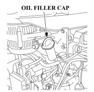
When the engine oil is contaminated or discolored, replace with the fresh engine oil (see page 90 for replacement interval and procedure).
