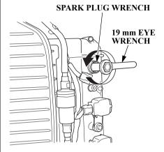
5. Use the spark plug wrench and 19 mm eye wrench to remove the spark plugs.
