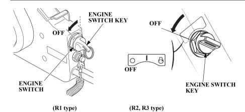
2. Turn the engine switch key to the OFF position to stop the engine.
