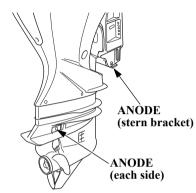
The anode is a sacrificial material which helps to protect the outboard motor from corrosion.
