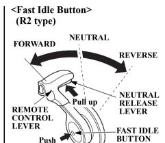
Pushing the fast idle button, turn the remote control lever forward. Keep turning the lever forward. The throttle opens and the engine speed increases after the lever passed the shift point. Note that the gearshift mechanism does not function when the fast idle button is pushed once and then released after the remote control lever is moved.
