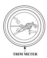
The trim meter has a range of  $-4^{\circ}$  to  $16^{\circ}$  and indicates the trim angle of the outboard motor. Refer to the trim meter when using the power trim/tilt switch to achieve proper boat performance.
