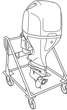
Transport and store the outboard motor either vertically, as shown above. Attach the stern bracket to stand and secure the outboard motor with bolts and nuts. Store the outboard motor in a well-ventilated area free from direct sunlight and humidity.
