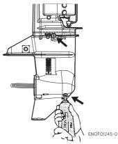
Install the upper oil plug, and then remove oil tube nozzle and install the lower oil plug. ENOW00095-0
