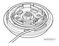
Tie a loop in the another end of the emergency starter rope and attach socket wrench that is included in the tool kit.
