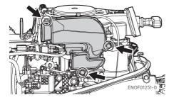
3. Remove starter lock cable from recoil starter by pulling the starter lock cable.
