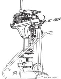
Keep the outboard motor in a vertical
