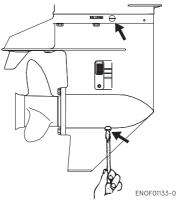
3. Insert the oil tube nozzle into the lower oil plug hole, and fill with gear oil by squeezing the oil tube until oil flows out of the upper plug hole and bubbles is disappeared to remove the air.
