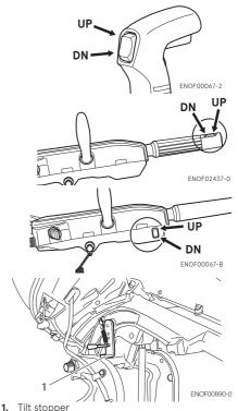
The outboard motor can also be tilted up and down using the switch provided under the bottom cowl.
