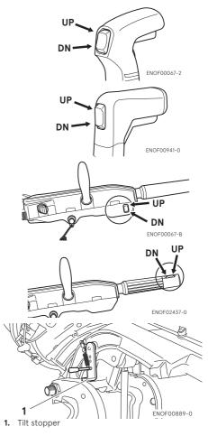
The outboard motor can also be tilted up and down using the switch provided under the bottom cowl.
