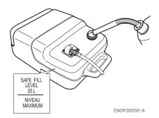
After filling the tank, close the fuel tank cap until two clicks sound is heard. ENOM00037-A
