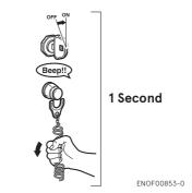
Within 5-10 seconds, Pull the red knob on the safety switch out and release.
