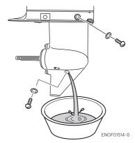
3. Insert the oil tube nozzle into the lower oil plug hole, and fill with gear oil by squeezing the oil tube until oil flows out of the upper plug hole and bubbles is disappeared to remove the air.
