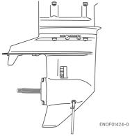
Insert the oil tube nozzle into the lower oil plug hole, and fill with gear oil by squeezing the oil tube until oil flows out of the upper plug hole and bubbles is disappeared to remove the air.
