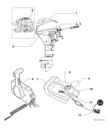
Warning label regarding owner's manual, top cowl, engine stop switch, engine oil level and unleaded gasoline.
