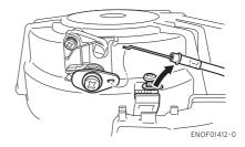
3. Remove the bolts (3 pcs) and remove the recoil starter.
