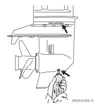
4. Install the upper oil plug, and then remove oil tube nozzle and install the lower oil plug.
