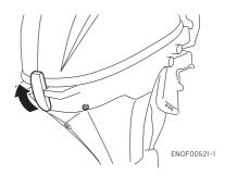
Remove starter lock cable from recoil starter by loosening the screw for the starter lock cable.
