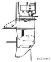
Insert the oil tube nozzle into the lower oil plug hole, and fill with gear oil by squeezing the oil tube until oil flows out of the upper plug hole and bubbles is disappeared to remove the air
