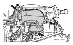
Remove starter lock cable from recoil starter by pulling the starter lock cable.
