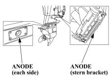
The anodes are located on each side of the gear case and on the stern bracket. They are made of a sacrificial material that helps to protect the outboard motor from corrosion.
