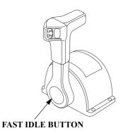
Use the fast idle button to accelerate engine warm-up after starting the engine. Do not use the fast idle button when starting the engine.
