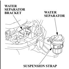
4. Remove the suspension strap from the water separator bracket; then remove the strap from the separator assembly.
