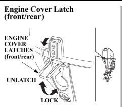
The engine cover latch fastens the engine cover to the outboard motor.
