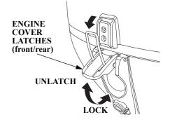
The engine cover latches fasten the engine cover to the outboard motor.
