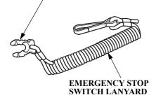
The emergency stop switch clip must be inserted in the emergency stop switch in order for the engine to start and run. The emergency stop switch lanyard must be attached securely to the operator or to the operator's PFD (Personal Flotation Device).
