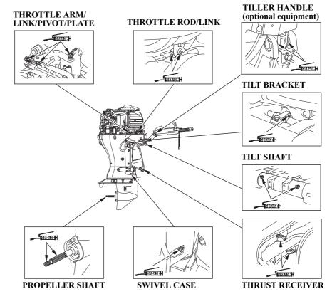
Apply corrosion inhibitor to all areas under the engine cover and any exposed metal surfaces except the belts.
