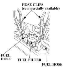
3. Before removing the fuel filter, to prevent fuel leakage, place fuel hose clips on the fuel hoses on each side of the fuel filter.
