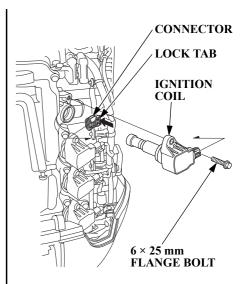
4. Remove the  $6 \times 25$  mm flange bolt. Disconnect the connector by pushing the lock tab and remove the ignition coil.
