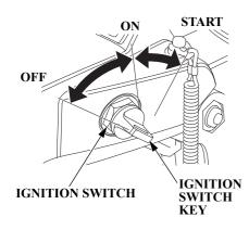
ON START OFF **IGNITION** SWITCH **IGNITION SWITCH** KEY The ignition switch controls the ignition system and the starter motor. Turning the ignition switch key to the START position operates the starter motor. The key automatically returns to the ON position when released from the START position. The engine will not start unless the gearshift lever is in the N (neutral) position (p. 68) and the emergency
