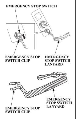
The emergency stop switch clip must be inserted in the emergency stop switch in order for the engine to start and run. The emergency stop switch lanyard must be attached securely to the operator or to the operator's PFD (Personal Flotation Device).
