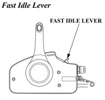
Use the fast idle lever to accelerate engine warm-up after starting the engine. Do not use the fast idle lever when starting the engine.
