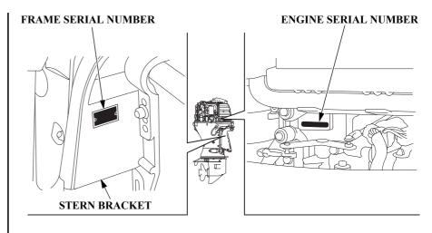
The frame serial number is stamped on a plate attached on the right side of the stern bracket.
