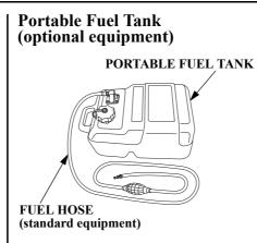
The portable fuel tank has a capacity of 6.6 US gal (25 L) and has a fuel gauge built into the fuel tank connector.
