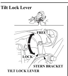
The tilt lock lever is used to support the outboard motor in the fully-raised position.
