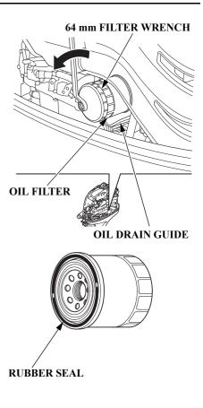
4. Clean the oil filter mounting base, and coat the rubber seal of the new oil filter with clean engine oil.
