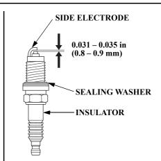
7. Measure the spark plug electrode gap with a wire-type feeler gauge. Correct the gap, if necessary, by carefully bending the side electrode. The gap should be: 0.031 - 0.035 in (0.8 - 0.9 mm)
