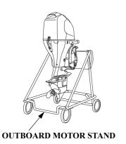
If the outboard motor will be removed from the boat for storage, we recommend storing it vertically by mounting it on a commercially available stand.
