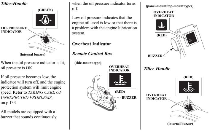
When the alert triggers, the overheat indicator comes on and the buzzer sounds a steady tone as the engine speed is reduced to 1,800 rpm. If the condition persists for another 20 seconds, the engine shuts off. Refer to *TAKING CARE OF UNEXPECTED PROBLEMS*, on p.134.
