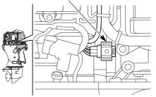
The NMEA2000<sup>®</sup> interface coupler can provide information regarding engine speed, fuel consumption, and various warnings to an existing NMEA2000 network via an optional interface cable. Contact your dealer for more information.
