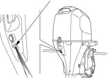
If overheating activates the engine protection system, idle the engine in neutral, and check the cooling system indicator.
