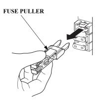
4. Use the fuse puller from the tool kit to remove the fuses. If a fuse is blown, install a replacement fuse of the same specified rating. The outboard motor is supplied with spare fuses in the fuse holder.
