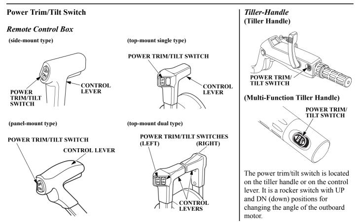
You can use the power trim/tilt switch anytime whether the boat is underway, stopped, or the ignition switch is in the OFF position. It is necessary for the ignition switch to be in the ON position for the trim meter to indicate the outboard motor angle. Trim the outboard motor to obtain the best performance and stability (p.81).
