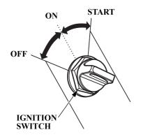
The ignition switch controls the ignition system and the starter motor.
