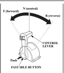
The fast idle button allows you to increase the idle speed without engaging the drive gears. Move the control lever toward the F (forward) or R (reverse) position after pushing in the fast idle button to increase the idle speed. It is necessary to position the control lever in the N (neutral) position to push in the fast idle button.
