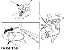
Adjust the trim tab with the engine stopped. Remove the gear case grommet. Loosen the trim tab bolt above the trim tab, turn the trim tab, and then tighten the bolt and install the gear case grommet securely. When the trim tab is correctly adjusted, steering effort will be equal in both directions.
