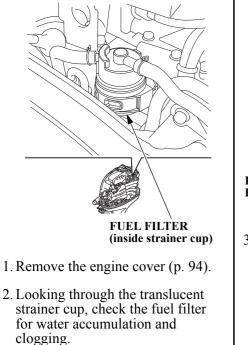
If necessary, replace the fuel filter with a new one.
