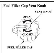
The fuel filler cap is provided with a vent knob to seal the portable fuel tank for carrying it to and from the boat. Open the vent by turning the vent knob counterclockwise all the way before starting the engine.
