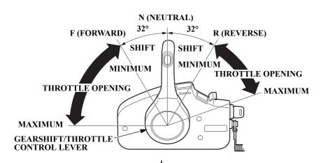
Moving the control lever 32° from N (neutral) selects the gear, and further movement increases engine speed.
