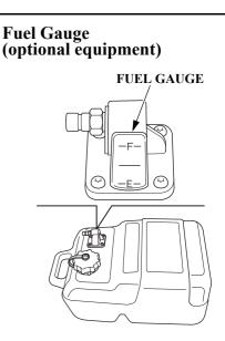
A fuel gauge is built into the fuel tank connector of the portable fuel tank.
