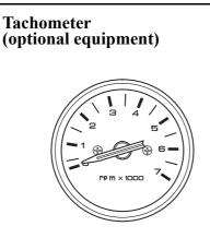
The tachometer shows engine speed in revolutions per minute.
