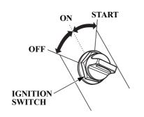
The ignition switch controls the ignition system and the starter motor.
