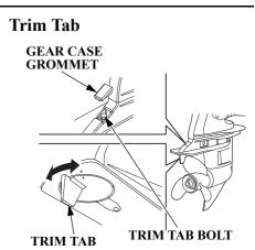
The trim tab compensates for "torque steer," which is a reaction of the outboard motor to propeller rotation.
