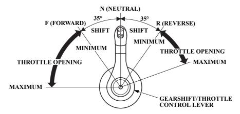
Moving the control lever 35° from N (neutral) selects the gear, and further movement increases engine speed.
