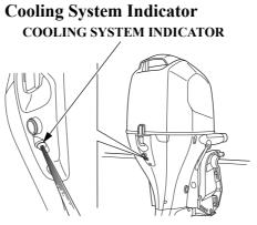
Water should flow from the cooling system indicator while the engine is running. This shows that water is circulating through the cooling system.
