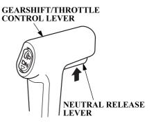
The gearshift/throttle control lever controls engine speed and selects F (forward), N (neutral), or R (reverse) gears.
