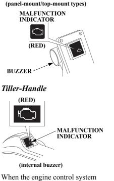
detects an engine control system malfunction, the malfunction indicator turns on and the buzzer sounds at one-second intervals.
