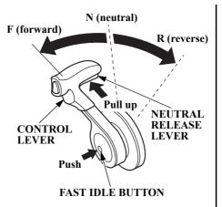
The fast idle button allows you to increase the idle speed without engaging the drive gears. Move the control lever toward the F (forward) or R (reverse) position after pushing in the fast idle button to increase the idle speed. It is necessary to position the control lever in the N (neutral) position to push in the fast idle button.
