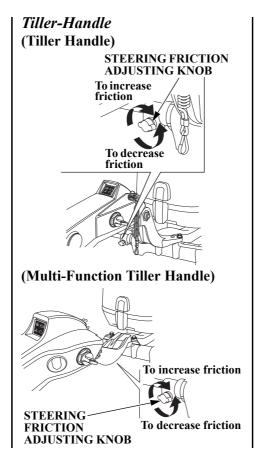
Tighten the steering friction adjusting knob securely.
