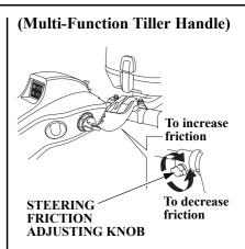
Use the steering friction adjusting knob to adjust the tiller handle friction. Turning it clockwise increases friction and turning it counterclockwise decreases friction.
