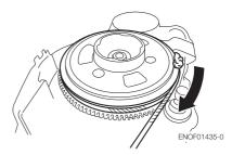
5. Tie a loop in the another end of the emergency starter rope and attach socket wrench that is included in the tool kit.
