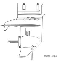
Insert the oil tube nozzle into the lower oil plug hole, and fill with gear oil by squeezing the oil tube until oil flows out of the upper plug hole and bubbles is disappeared to remove the air.
