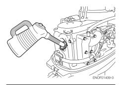
Use only high quality 4-stroke engine oil to insure performance and prolonged engine life.
