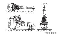
Keep the outboard motor in a vertical position when carrying.
