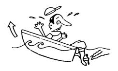
■ Improper Trim Angle (bow dips into the water)
