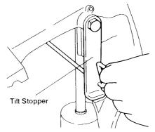
(B) Return to normal running position Move (UP) lock lever to "Free" position. Outboard motor moves down to thrust rod. Move (DOWN) lock lever to "Lock" position.
