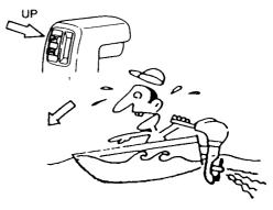
■ Proper Trim Angle The trim angle is optimum when the boat is parallel to the water surface while running.
