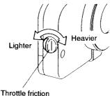
Throttle friction adjustment screw
