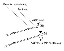
② Fitting of Remote Control Cable to Engine
