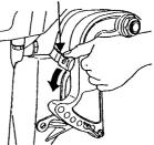
(2) Return to normal running position:Put the reverse lock lever in the tilt down position, slightly lift up the engine, and then put it down.
