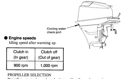
Propeller must be selected that will allow the engine to reach recommended rpm when cruising at wide-open throttle.
