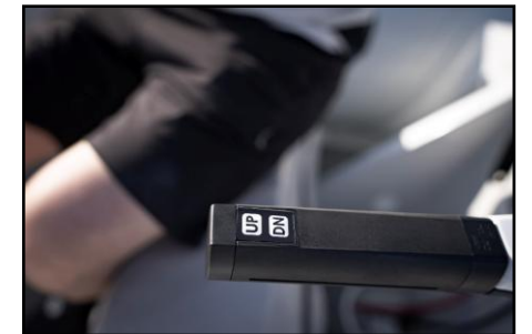
Integrated Power Trim & Tilt Switch at Tiller Handle Grip
