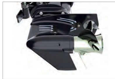
Auxiliary Water Intake Port
