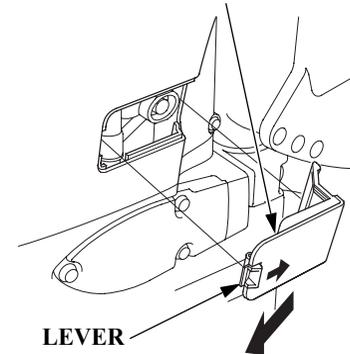
2. Push the drain bolt cover lever and remove the cover while pulling the cover backward at an angle.
