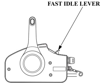
Use the fast idle lever to accelerate engine warm-up after starting the engine. Do not use the fast idle lever when starting the engine.
