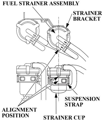
8. Align the center of suspension strap with the screw position and install the fuel strainer assembly.
