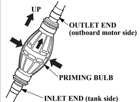
A priming bulb is built into the fuel hose that connects the fuel tank to the outboard motor.
