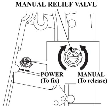
The outboard motor can be tilted manually after opening the manual relief valve. This allows the outboard motor to be tilted up or down when no battery is connected.
