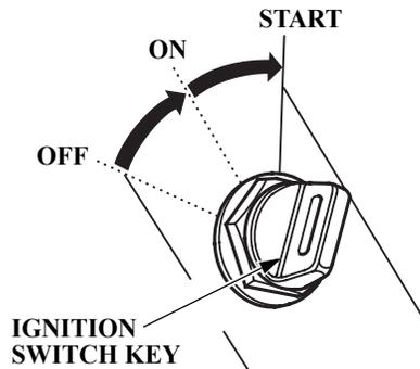
3. Turn the ignition switch key to the ON position; the buzzer will sound twice.
