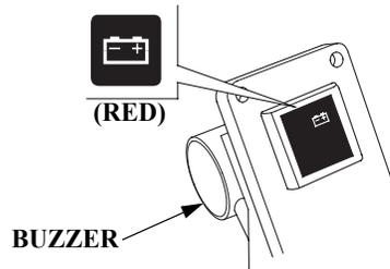
The ACG indicator turns on and the buzzer sounds in one-second intervals when the charging system is faulty.
