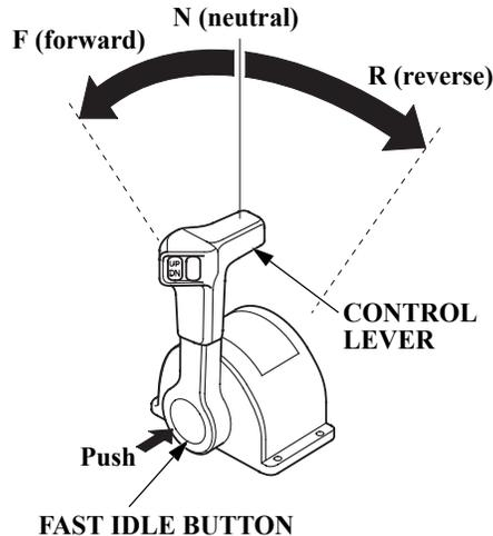
The fast idle button allows you to increase the idle speed without engaging the drive gears. Move the control lever forward or reverse after pushing in the fast idle button to increase the idle speed.
