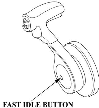
Use the fast idle button to accelerate engine warm-up after starting the engine. Do not use the fast idle button when starting the engine.
