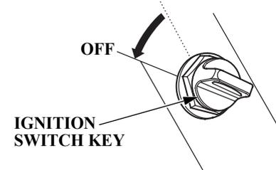
2. Turn the ignition switch key to the OFF position to stop the engine. In the event that the engine does not stop when the ignition switch key is turned to OFF, press the emergency stop switch until the engine stops.
