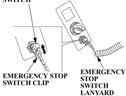
1. Put the emergency stop switch clip in the emergency stop switch, and attach the emergency stop switch lanyard securely to the operator or to the operator's PFD (Personal Flotation Device).
