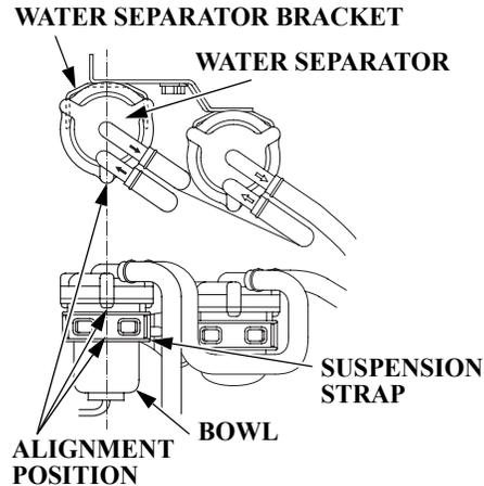
7. Align the center of suspension strap with the screw position and install the water separator assembly.
