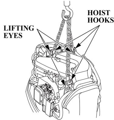
2. Attach the hoist hooks to the lifting eyes.
