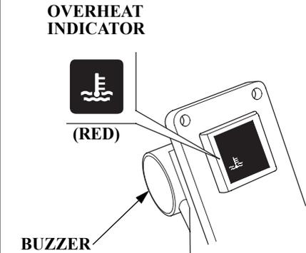
When the alert triggers, the overheat indicator comes on and the buzzer sounds a steady tone as the engine speed is reduced to 1,800 rpm. If the condition persists for another 20 seconds, the engine shuts off. Refer to *TAKING CARE OF UNEXPECTED PROBLEMS*, on p. 101.
