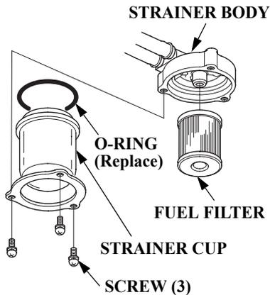
5. Remove the three screws and separate the fuel strainer cup from the strainer body.
