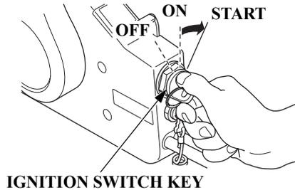
4. Turn the ignition switch key to the ON position; the buzzer will sound twice.
