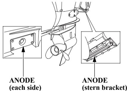
The anodes are made of a sacrificial material that helps to protect the outboard motor from corrosion.
