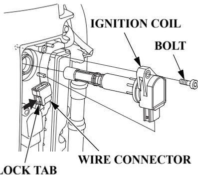
6. Use a 6 mm hex. wrench to remove the bolt holding the ignition coil. Move the ignition coil to a position that allows removal of the wire connector easily.
