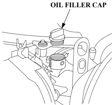
4. If the oil level is low, remove the oil filler cap, and add oil to reach the upper limit mark shown on the dipstick. Use the oil recommended on p. 70.
