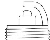
10. Inspect the spark plugs. Replace them if the electrodes are worn, or if the insulators are cracked or chipped.
