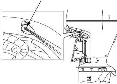
If overheating activates the engine protection system, idle the engine in neutral, and check the cooling system indicator.
