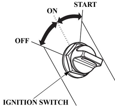
The ignition switch controls the ignition system and the starter motor.
