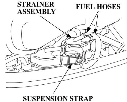
3. Remove the strainer assembly. If it is difficult to remove the strainer assembly by yourself, consult an authorized TOHATSU dealer. Remove the suspension strap from the fuel filter bracket, and then remove the strap from the fuel filter assembly.
