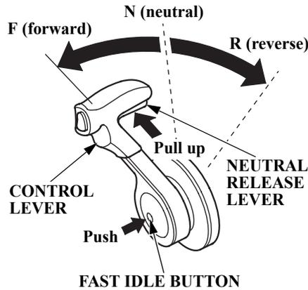
The fast idle button allows you to increase the idle speed without engaging the drive gears. Move the control lever forward or reverse after pushing in the fast idle button to increase the idle speed.
