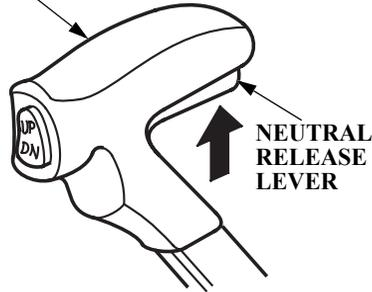
The gearshift/throttle control lever controls engine speed and selects F (forward), N (neutral), or R (reverse) gears.
