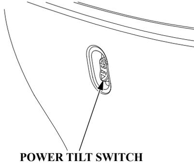
The power tilt switch is located on the engine pan. It is a rocker switch with UP and DN (down) positions for changing the angle of the outboard motor.
