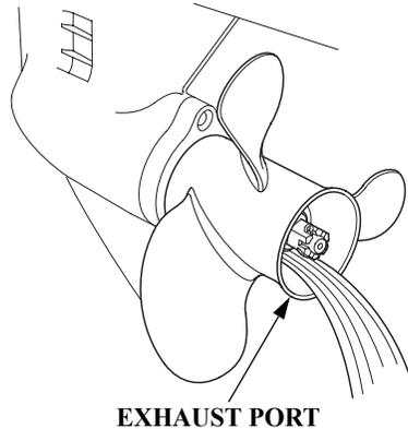
6. Turn on the fresh water supply and flush the outboard motor for at least 10 minutes.
