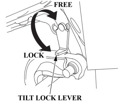
The tilt lock lever is used to support the outboard motor in the fully-raised position.
