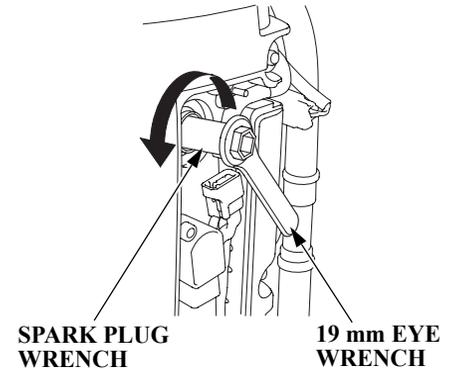
9. Remove the spark plugs with a spark plug wrench and 19 mm eye wrench.
