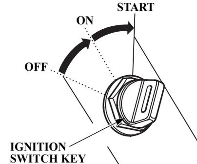
3. Turn the ignition switch key to the ON position; the buzzer will sound twice.
