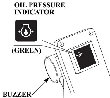
When the oil pressure indicator is lit, oil pressure is OK.
