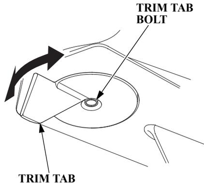
The trim tab compensates for “torque steer,” which is a reaction of the outboard motor to propeller rotation.
