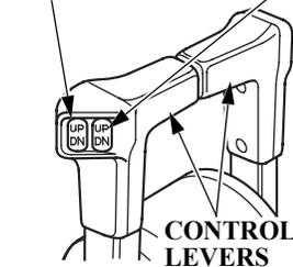
The power trim/tilt switch is located on the control lever. It is a rocker switch with UP and DN (down) positions for changing the angle of the outboard motor.
