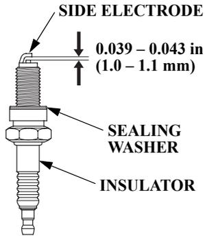
11. Measure the spark plug electrode gap with a wire-type feeler gauge. Correct the gap, if necessary, by carefully bending the side electrode.
