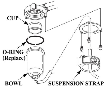
4. Remove the three screws and separate the bowl from the body.
