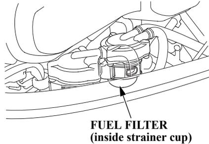
2. Looking through the translucent strainer cup, check the fuel filter for water accumulation or sediment.
