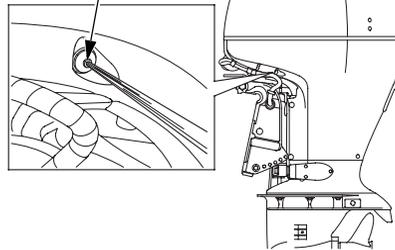
Water should flow from the cooling system indicator while the engine is running. This shows that water is circulating through the cooling system.
