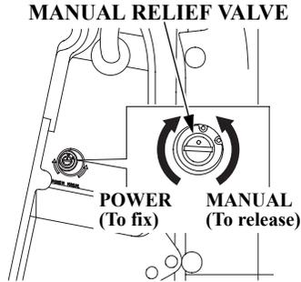
The outboard motor can be tilted manually after opening the manual relief valve. This feature enables the outboard motor to be tilted up or down when no battery is connected.
