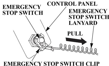
To stop the engine in an emergency, pull the emergency stop switch clip out of the emergency stop switch by pulling the emergency stop switch lanyard.
