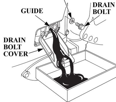
4. Place a suitable container below the oil drain guide to catch the used oil, and then remove the oil filler cap, drain bolt, and sealing washer.
